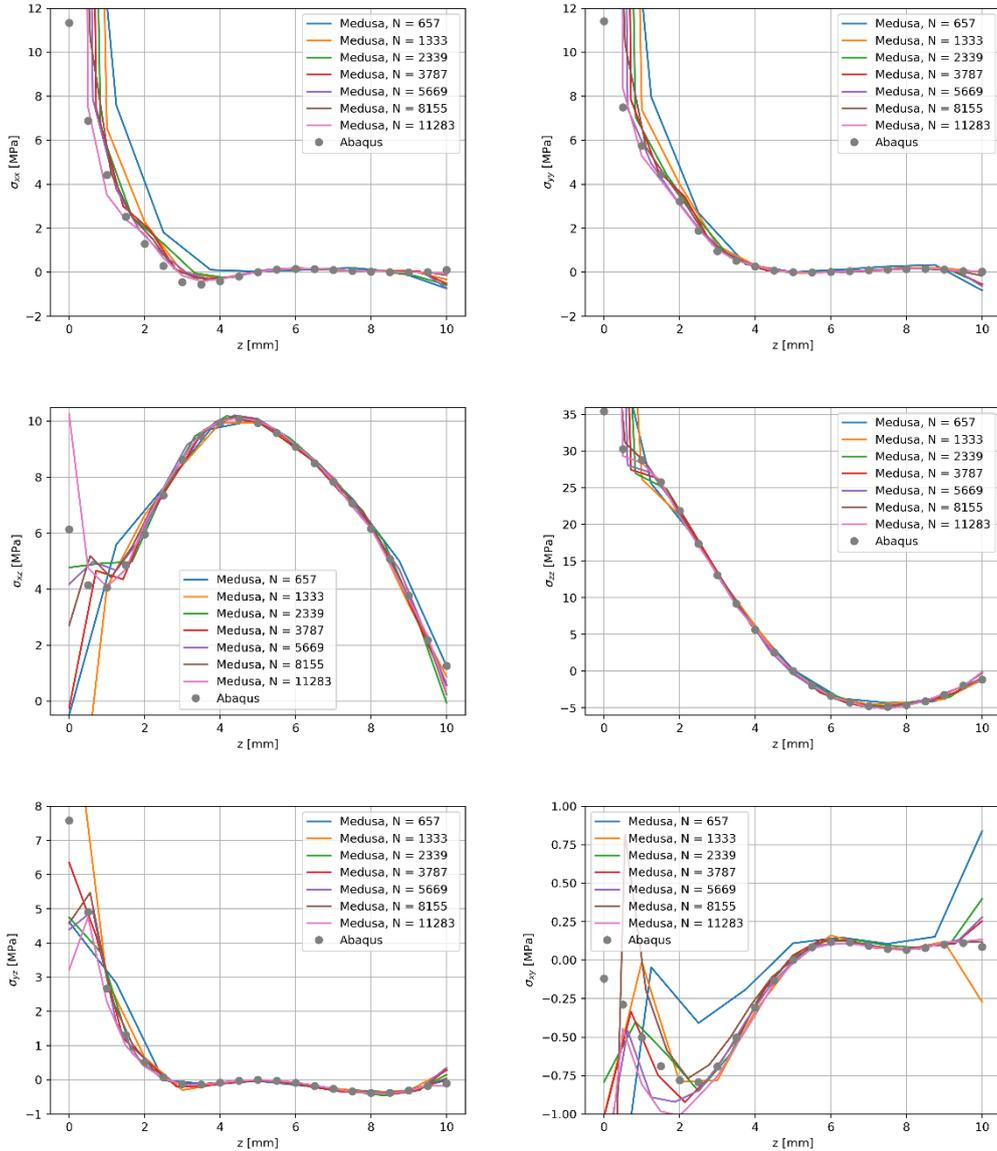
Figure 4: Results of meshless WLS (Medusa) computations (solid lines) vs. Abaqus (grey dots).  $N$  is the number of discrete points in the domain. Displayed are the six components of the stress tensor  $\sigma$ , clockwise starting from top left:  $\sigma_{xx}$ ,  $\sigma_{yy}$ ,  $\sigma_{zz}$ ,  $\sigma_{xy}$ ,  $\sigma_{yz}$ ,  $\sigma_{xz}$ .
