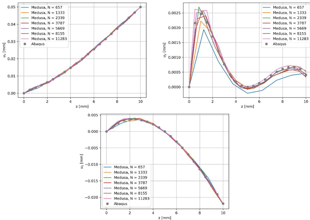
Figure 3: Results of meshless WLS (Medusa) computations (solid lines) vs. Abaqus (grey dots).  $N$  is the number of discrete points in the domain. Displayed are the three components of displacement  $\mathbf{u}$ , clockwise starting from top left:  $u_x$ ,  $u_y$ ,  $u_z$ .
