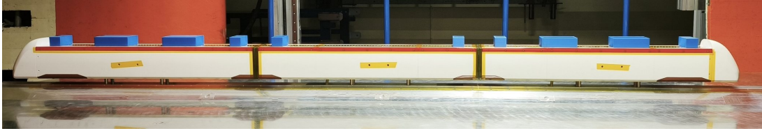
Figure 11: KMF-Regio model in scale 1:25, equipped with reference roof boxes (config. 10) as mounted in the test section of 3m-LSWT
