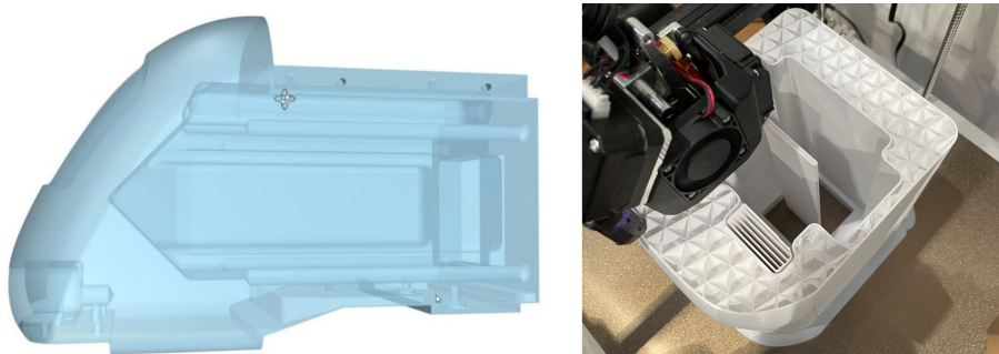
Figure 5: The trains head as prepared for 3D printing: left) transparent view of the part in CAD, right) head being printed on a conventional filament printer
