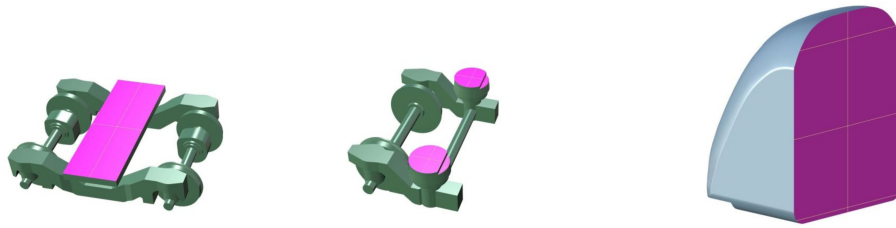
Figure 3: Interface surfaces to be used for own designs of bogies and train heads (purple areas): single-car bogies (left), Jacobs bogies (middle) and heads (right)
