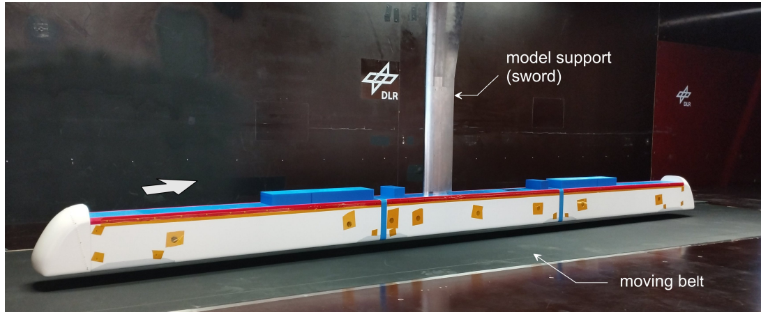
Figure 6: KMF-Regio scale 1:20 model as mounted in the SWG wind tunnel
