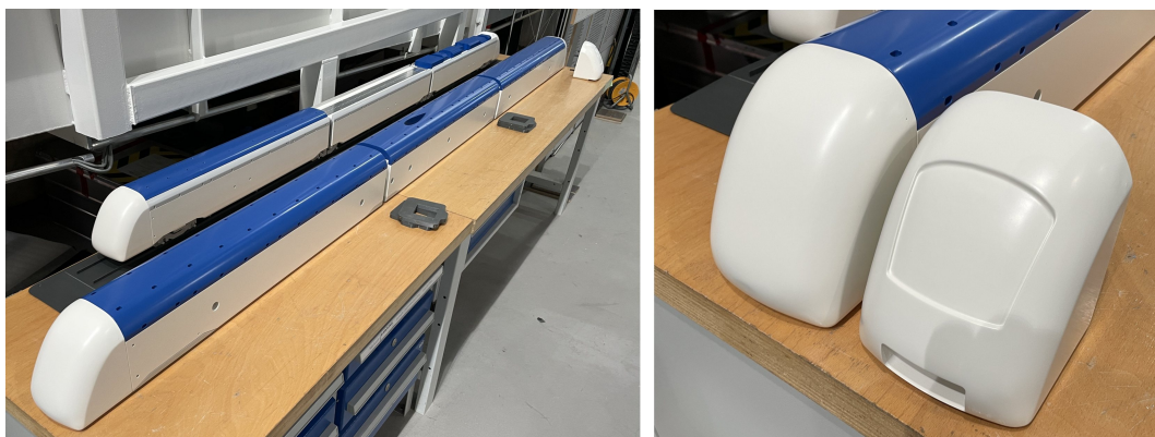
Figure 9: Comparison of scale 1:25 to 1:20 model (left) and comparison of smooth head to realistic head (right: realistic head w/o coupler and snow plow)
