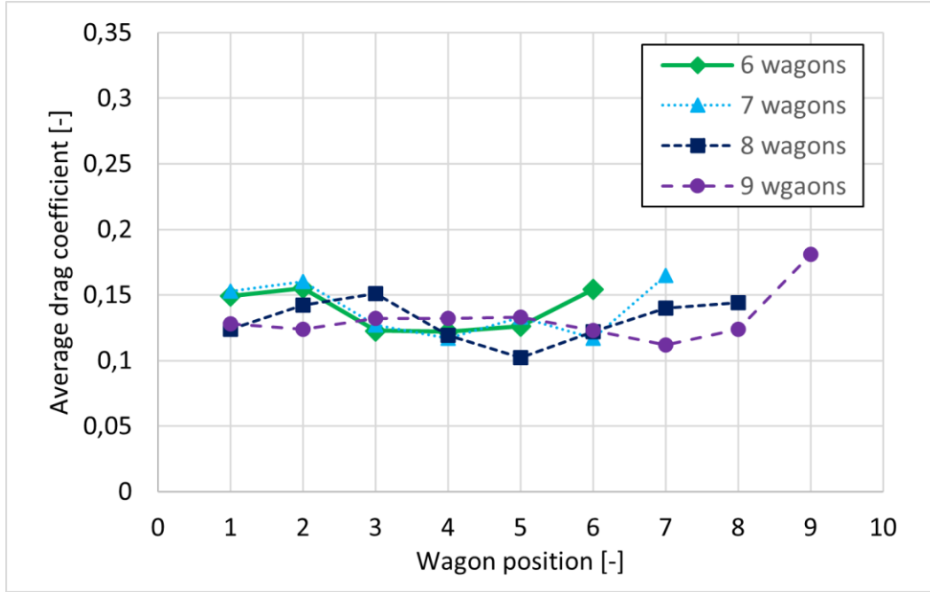
Figure 3. Average drag coefficients on downstream containers in all tested train compositions
