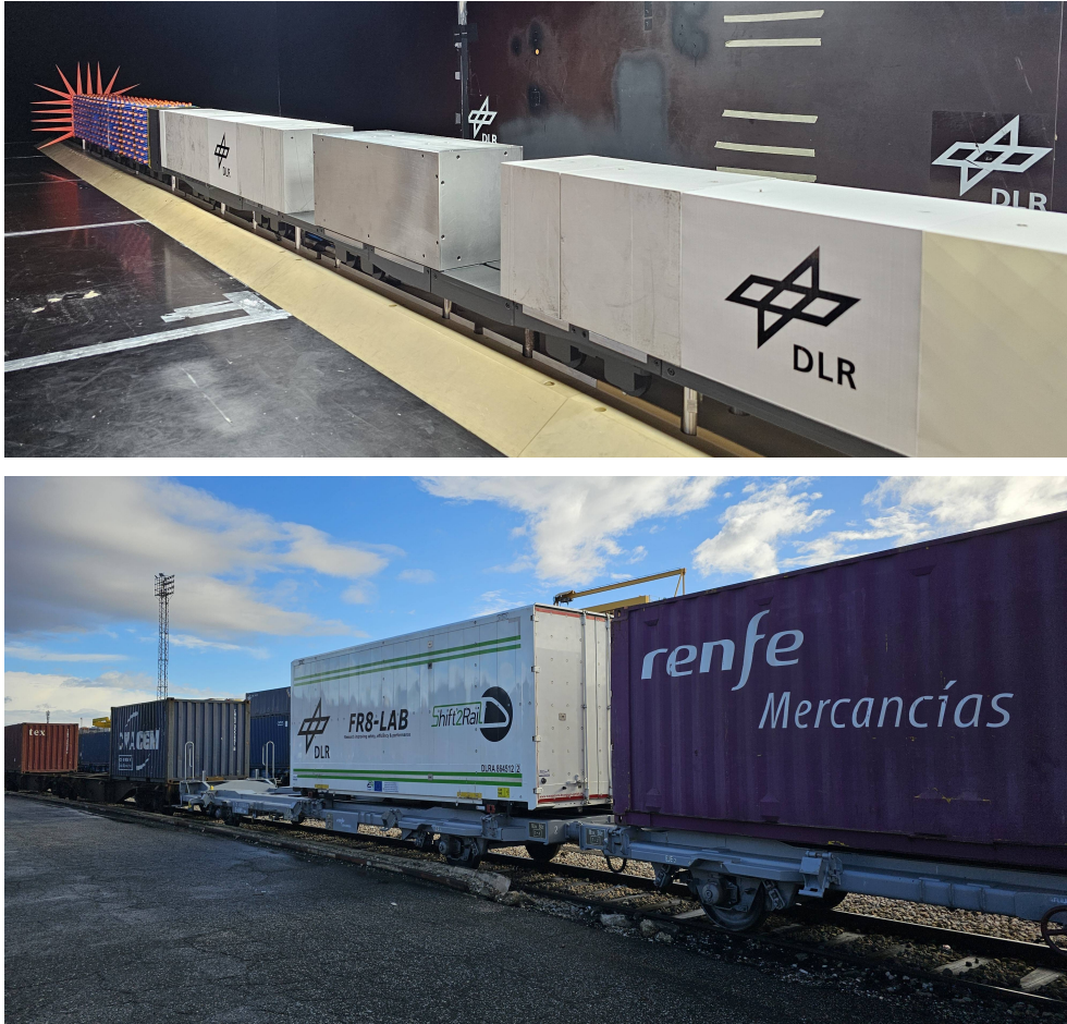
Figure 1: Wind-Tunnel experiment model, at 1:15 scale, with a FR8-LAB test-container, representative gap in front and detailed generic wagon geometry (above) DLR FR8-LAB during field measurements on operational freight-trains in Spain, used as validation for the wind-tunnel methodology developed in the presented work (below).
