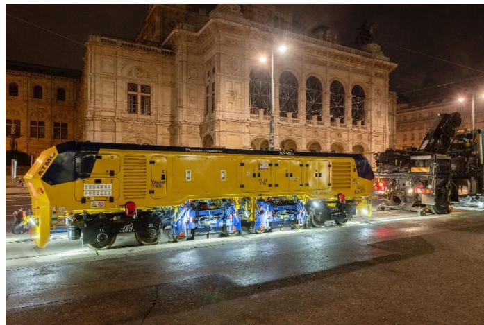
Figure 1: Urban rail grinding trailer ATMO (Automated Track Machine Oscillator) towed by a high-rail vehicle.
