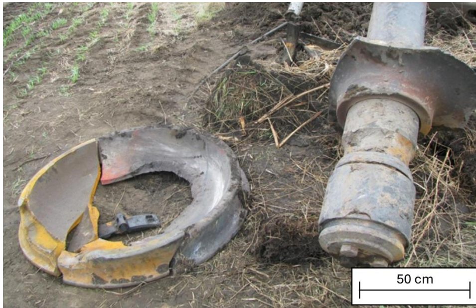
Figure 1: Fractured wheel remnants, photographed at the accident site.
