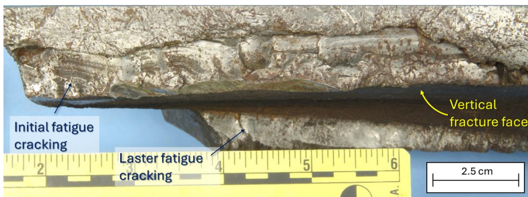
Figure 4: The subsurface (initial) progressive cracking viewed from the tread surface
