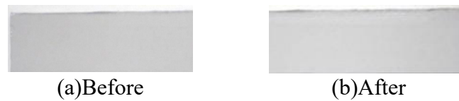
Figure 12: Appearance of Test Specimens Before and After the Weather Resistance Test
