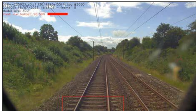
Figure 4: Using a ‘letterbox’ approach to hone in on relevant track for the low ballast classifier model
