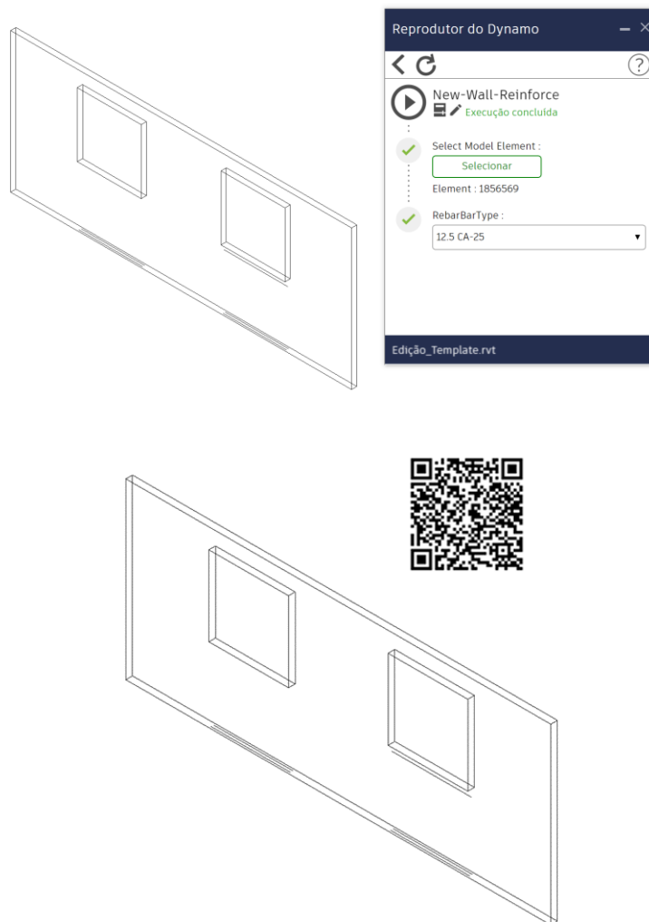
Figure 19: Execution of reinforcement in windows, with data and output input.
