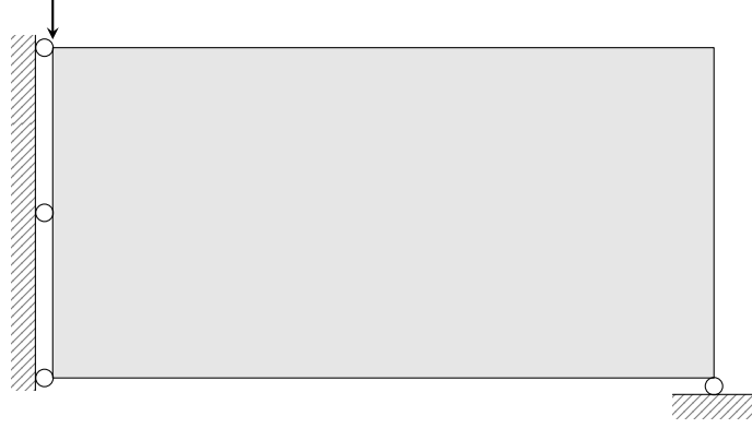
Figure 3: Design domain, load, and boundary conditions of the MBB beam benchmark. The left edge is fixed horizontally, the bottom-right corner vertically, and a downward load acts at the upper-left corner.
