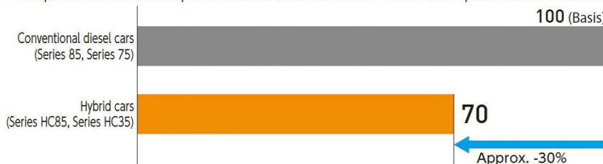
Figure3: Comparison of diesel fuel consumption of conventional diesel cars (Series 85, Series 75) and hybrid cars (Series HC85, Series HC35).
