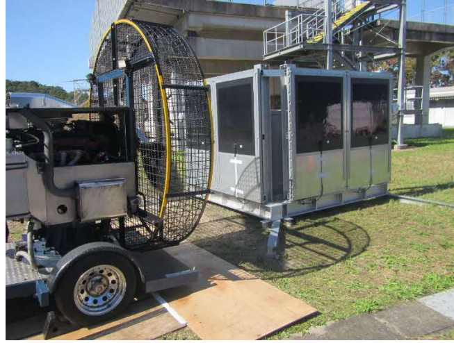
Figure 15: Wind-pressure testing setup for prototype sound-barrier units.
