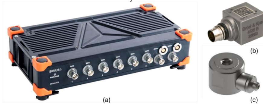
Figure 2: Equipment used during the test: Data acquisition system (a), accelerometer (b) and hammer force sensor (c)
