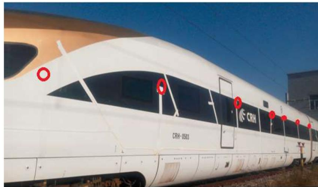
Figure 6: Modal test in field line
