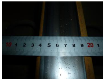
Figure 8: Rail absence of grinding
