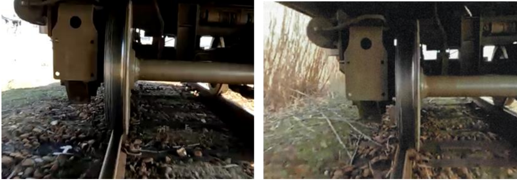
Figure 13: Examples of images captured during mainline operations. (Left : The whole area of the rail top surface is covered by the wheel Right : The partial area of the rail top surface is covered by the wheel)
