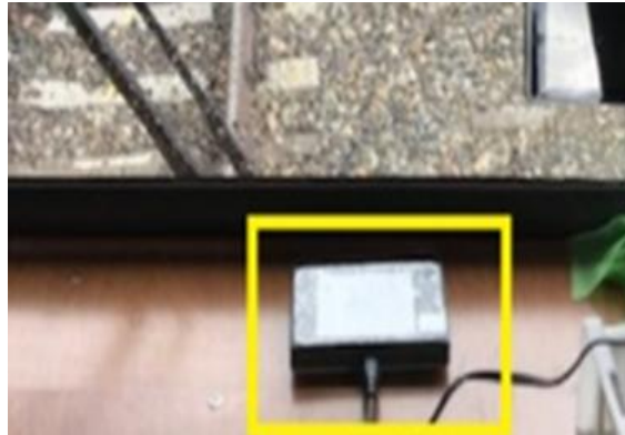
Figure 2: Measurement of vehicle vibration by using a compact device.
