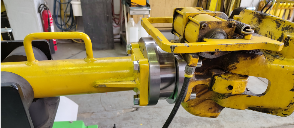
Figure 6: Mounted load cell in shunting coupling
