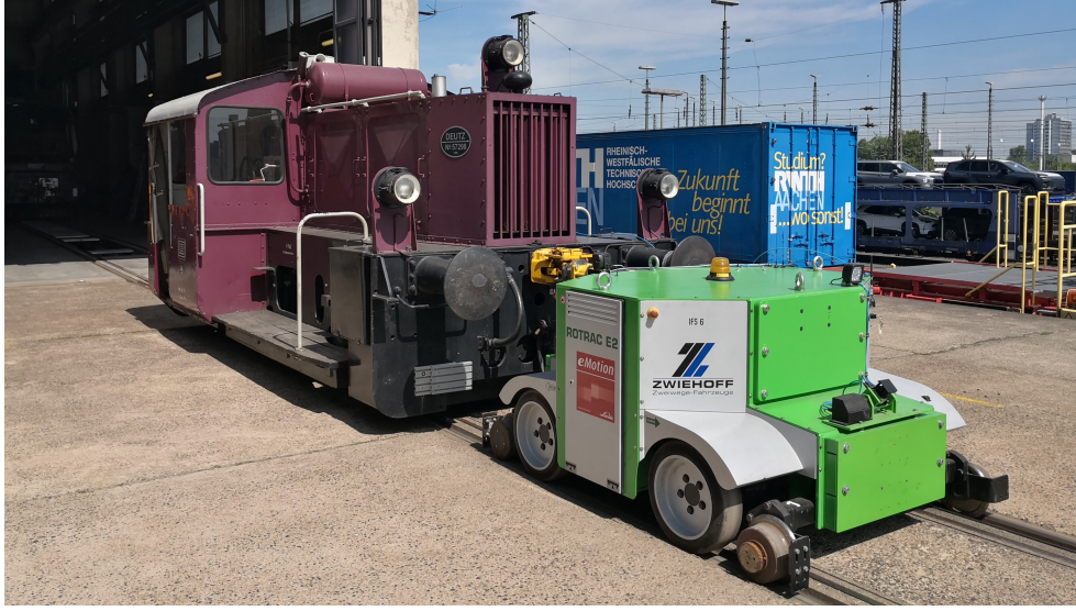
Figure 7: Experiment setup consisting of shunting locomotive Köf and road-rail vehicle Rotrac E2
