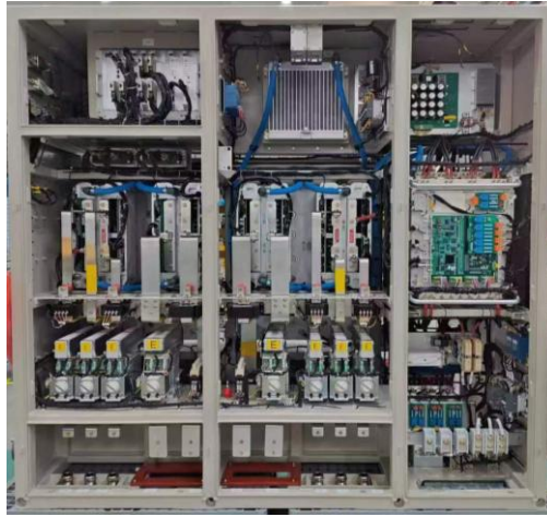
Figure 2: Silicon carbide traction converter and high-frequency auxiliary converter.
