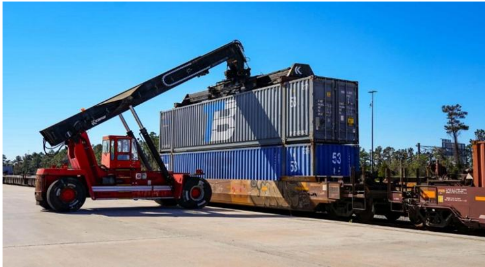
Figure 2: Illustration of the simplicity of the infrastructure needed for handling containers on trains
