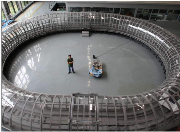
Fig 2. Ring-type HTS maglev test line. [11]
