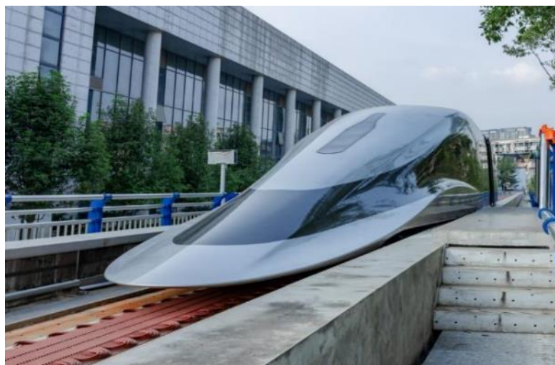
Fig 3. High-speed HTS maglev engineering prototype vehicle and test line.
