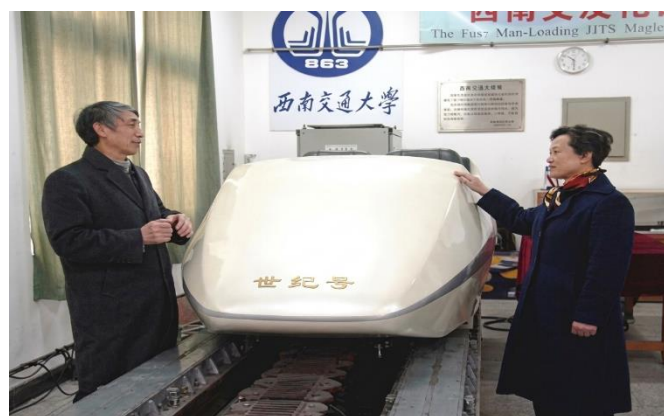
Fig 1. The world's first manned HTS maglev prototype vehicle.
