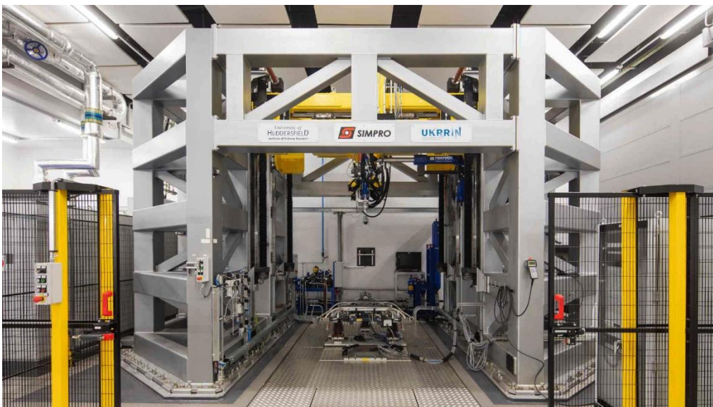
Figure 1: Full-scale pantograph test bench at the University of Huddersfield.
