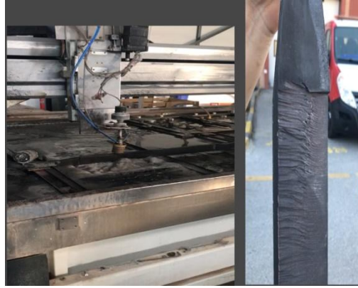
Figure 2: Rough surface profile of a scrap carbon strip after abrasive added water jet cutting at 4000 MPa. (Jet-leg effect was seen on the cutting surface and penetration is weak in transverse cutting direction)
