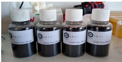
Figure 7: Graphite powder samples bottled in different mesh sizes, nominal 50-100 microns by Grafitor LLC.
