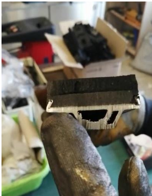
Figure 10: The cross section of coated graphite surface layer after running out of the scrap carbon strip surface manufactured by SHUNK Hoffman Co Company. (Black layer: Later filled surface layer and bottom gray layer: Original graphite layer)
