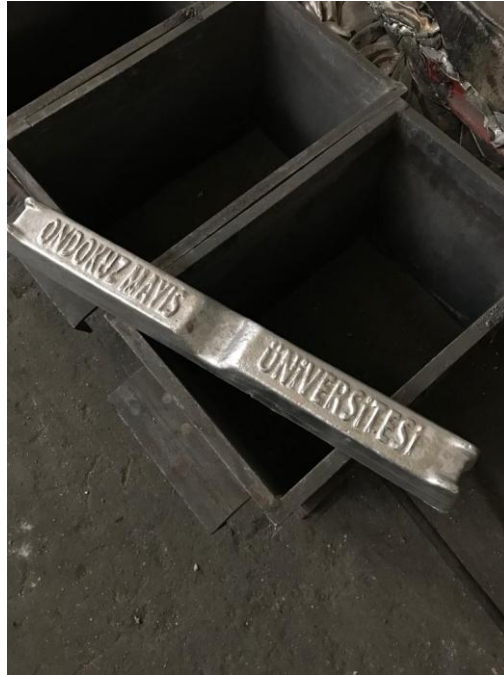
Figure 8: As-cast aluminum alloy ingot from the scrap aluminum profile
