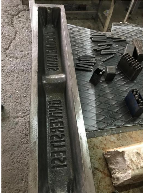
Figure 5: Melted aluminum alloy casting mold for ingot solidification
