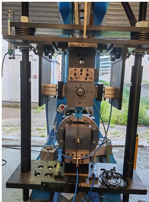
Figure 1: Twin disk test bench designed by PoliTo railway research team.
