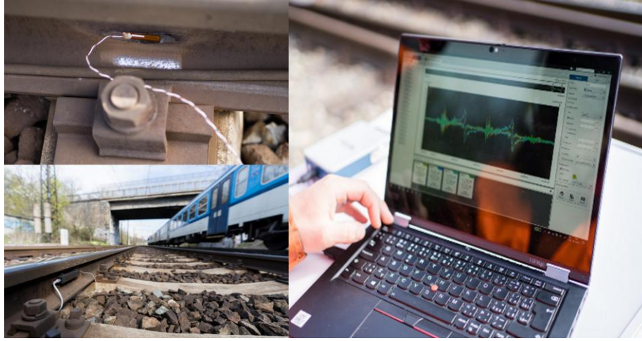
Figure 1: A piezoelectric MFC sensing element embedded on rail and output signal
