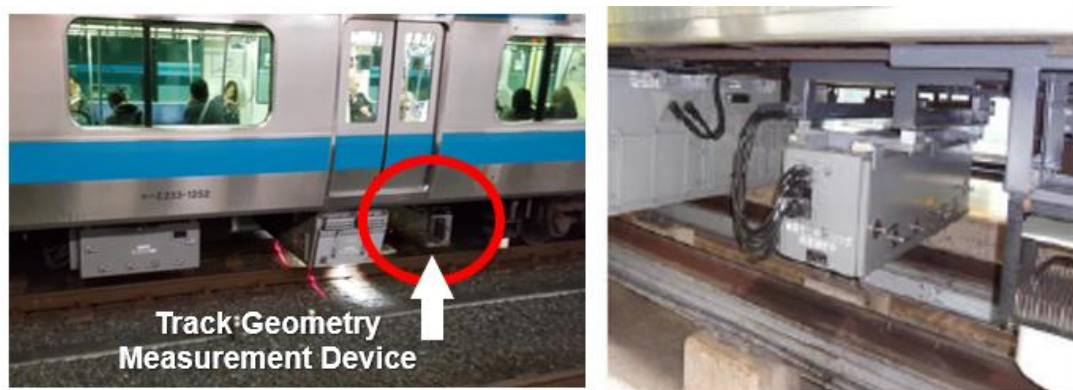
Figure 1: Track geometry measurement device.
