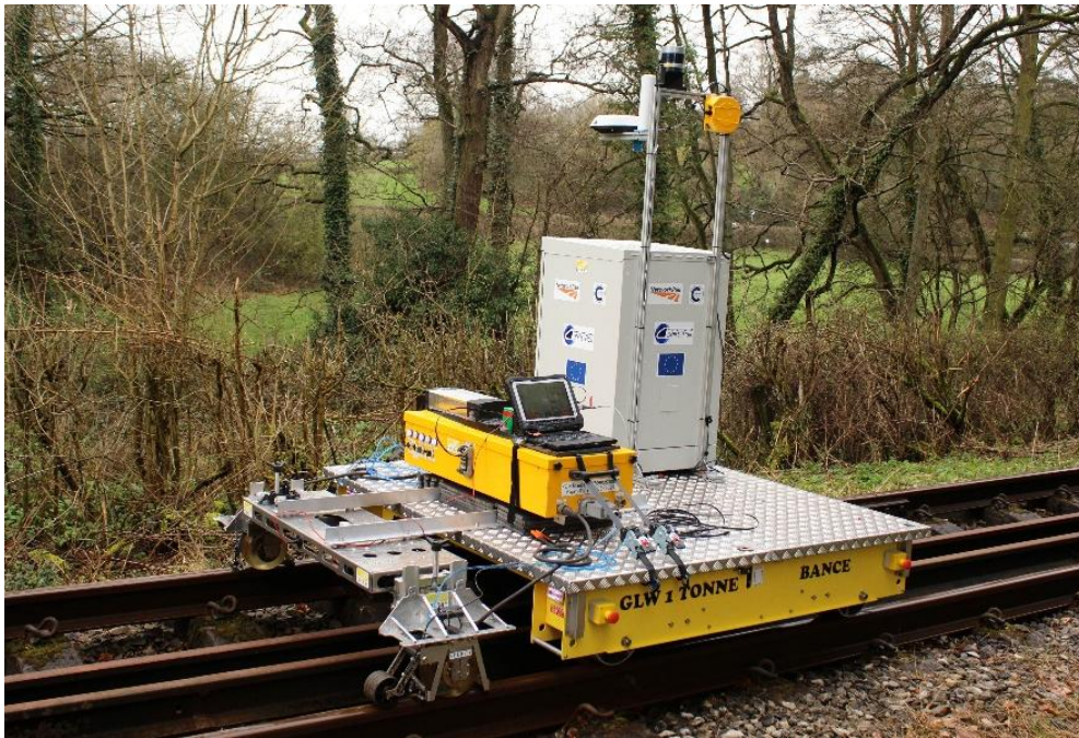
Figure 2: RIMV autonomous vehicle conducting a demonstration inspection at a heritage test railway.
