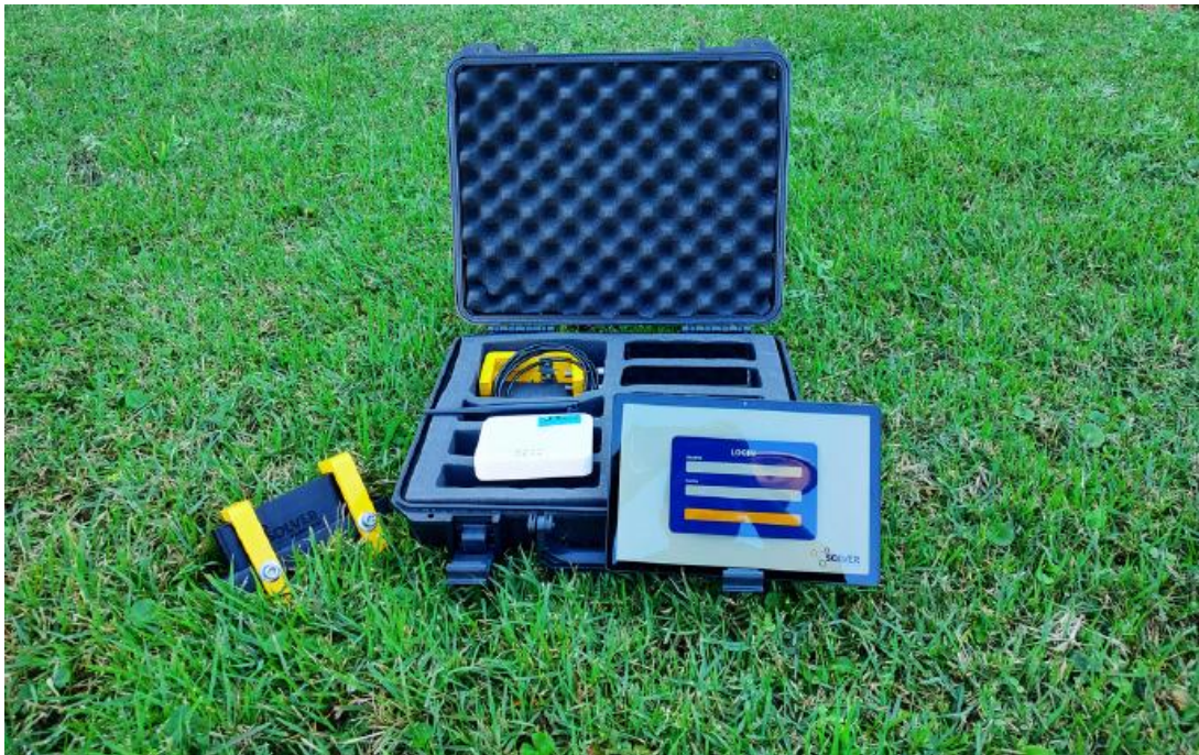
Figure 2: Portable instrumentation kit for field campaigns, containing ATT sensors, mechanical clamps, mini gateway, and the mobile management terminal.
