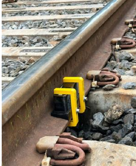
Figure 1: View of the ATT sensor coupled to the rail using the quick-release mechanical clamping system.
