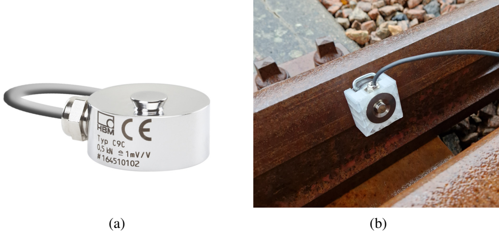
Figure 4: (a) Force load cell used in the measurements. (b) Square rig to hold the load cell. Additional spacers can be added to the rear of the load cell
