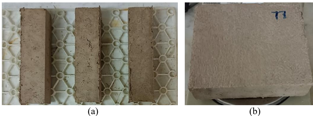
Figure 3. (a) Mechanical test samples, and (b) Thermal conductivity test sample.
