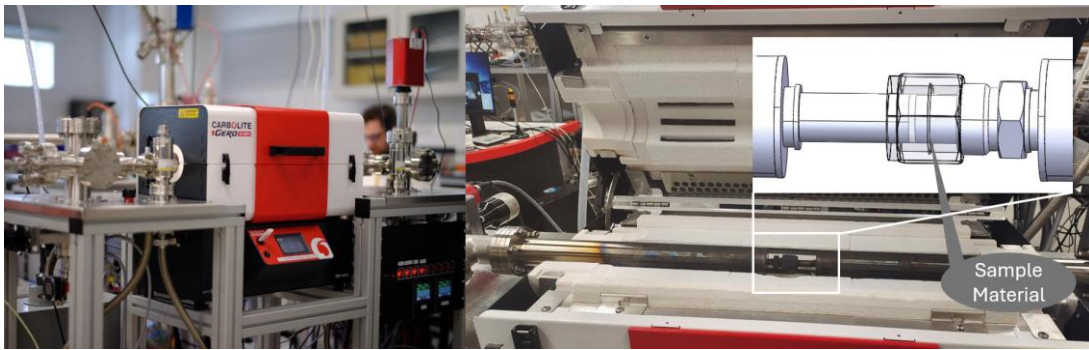
Figure 1: Gas-driven permeation system (left) and sample holder (right).
