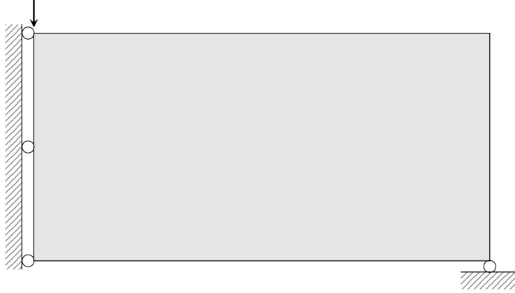
Figure 1: Design domain, boundary conditions, and external load for the MBB beam optimization problem.
