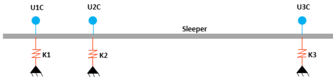
Figure 3 Simplified rail-sleeper-spring model.
